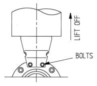
3. Using an allen key undo and remove the M6 cap screws. Loosen the screws a little at a time, diagonally at first as the valve halves separate. Once separated, remove the gasket / paddle / bottom cap assembly as shown.
