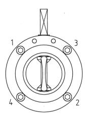
7. Replace the re-fitted spindle / seal assembly between the valve halves. Don't forget to replace the black plastic dust cap (if fitted). This fits between the valve halves at the base of the valve. Tighten the M6 bolts in a diagonal sequence as numbered in the illustration to the left, a little at a time. Ensure that all bolts are fully tight and that the valve halfs are fully tightened together. Place the valve in a vice and open and close the valve several times to ensure correct operation.
