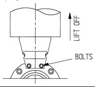
3. Using an allen key undo and remove the M6 cap screws. Loosen the screws a little at a time, diagonally at first as the valve halves separate. Once separated, remove the gasket / paddle / bottom cap assembly as shown. Place to one side.
