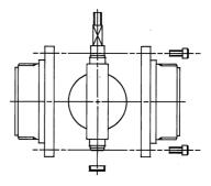
4. Prepare the pipe and valve ends for welding as per your company welding procedure and weld accordingly giving consideration to future maintenance access of the valve once welded in place. Once cooled, the valve can be re-assembled, noting correct bearing orientation as shown.
