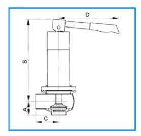
Designed to meet the changing needs of the process industry, the new Series 3 Pressure Relief valve uses elements of the DPL single seat valves to produce a full bore, self draining device ranging in size from 1-4".
