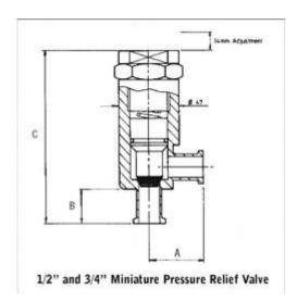
The 1/2" and 3/4" miniature PRV is available for applications not requiring a manual or actuated override. The Miniature PRV has a pressure range of 0.5 to 10 bar.
