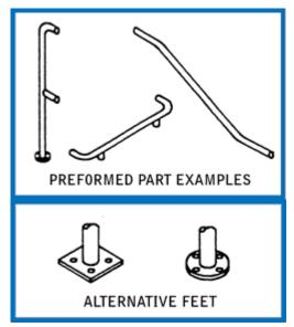
Handrail manufacture to customer specification or DPL design. Supplied as complete assembly, fully welded and polished or as preformed parts ready for on site assembly. Tube with prefabricated pullups or profiled ends for saddling. Square or round flange feet for base or wall mounting.
